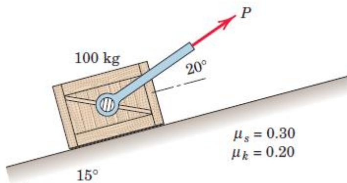
4. The magnitude of force  $P$  is slowly increased. Does the homogeneous box of mass  $m$  slip or tip first? State the value of  $P$  which would cause each occurrence. Neglect any effect of the size of the small feet.
