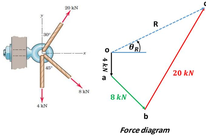
$\therefore R = \bar{oc} \times scale = 8.7 \times 2 = 17.4 \text{ kN}$
