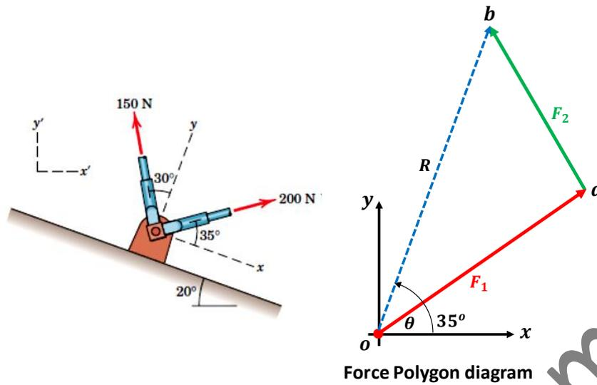
$$\therefore R = \overline{ob} \times \text{scale} = 10.3 \times 25 = 257.5 \text{ kN}$$
