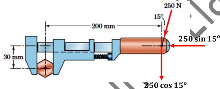
$$M = (250 \sin 15^\circ \times 30) - (250 \cos 15^\circ \times 200) = -46867.66 \text{ N.m} \curvearrowright$$
