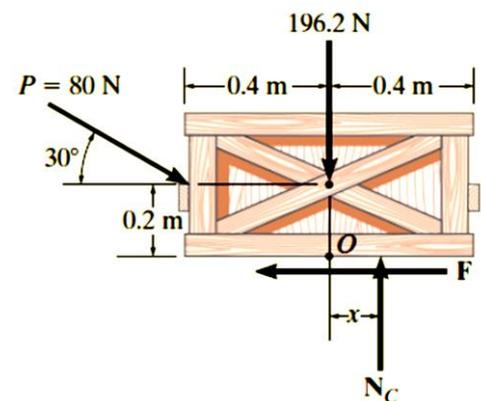
$$\therefore N_C = 236.2 \text{ N} \quad \text{and} \quad x = -0.00908 \text{ m} = -9.08 \text{ mm}$$
