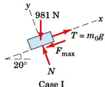
the plane, as shown in the free-body diagram of the block for **Case I** in the figure. With the weight  $mg = 100(9.81) = 981 \text{ N}$ , the equations of equilibrium give
