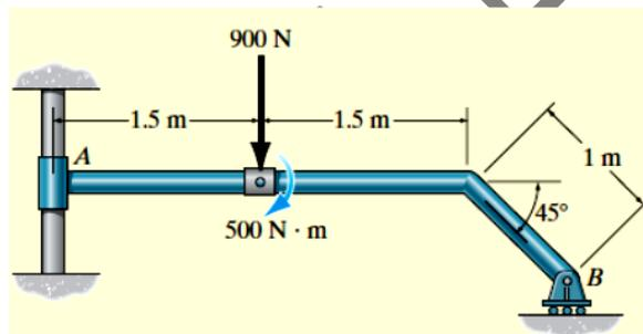
3. Determine the horizontal and vertical components of reaction on the beam caused by the pin at  $B$  and the rocker at  $A$  as shown in Figure. Neglect the weight of the beam.
