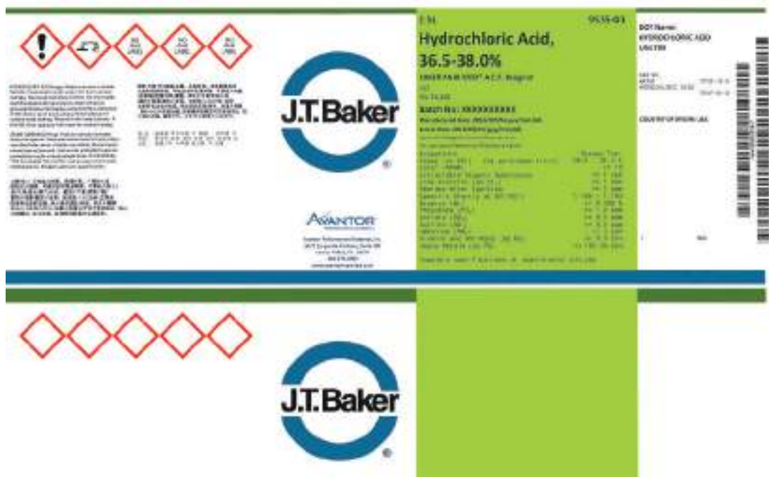
FIGURE 2-1 Label from a bottle of reagent-grade hydrochloric acid. Note that the specific gravity of the acid over the temperature range of 60° to 80°F is specified on the label. (Courtesy of Avantor Performance Materials, Radnor, PA.)
